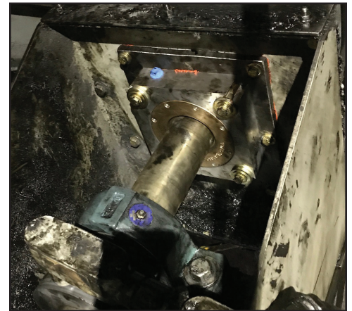
Air Mizer AM CEMA shaft seal installed on a CEMA Screw Conveyor.
